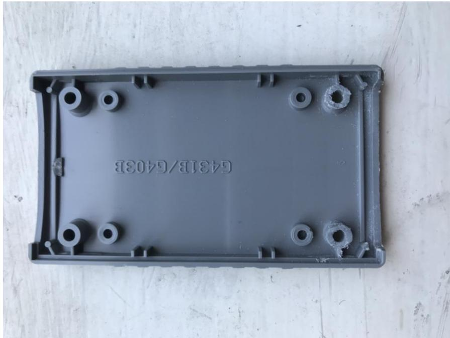
The picture above shows the other case half of the PIL Box that also needs the screw fixing posts to be reduced or removed to allow for the device connector.
