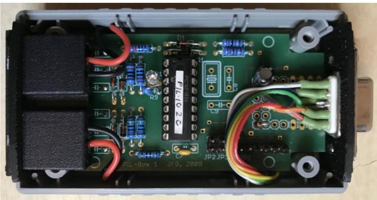
The picture above shows the 2 connectors installed in the PIO-IL housing. The IO pins on the PCB were a bit challenging to remove so the internal D type connector leads were soldered to the underside of the PCB.
