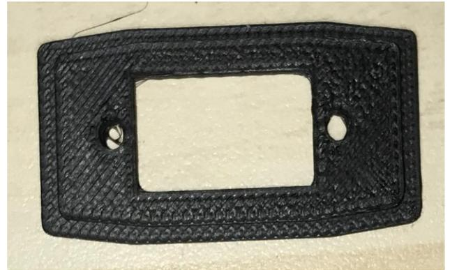
The pictures above show the 3D design that shows the step or 'lip' that fits in the PIL-IO housing groove and 2 fixing holes for the D type connector.
