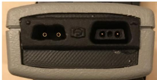
The pictures above show the 9 pin D connector mounted in the 3D end plate/housing and secured with 2 reclaimed screws (left) and the mounted HP-IL connector (right).
