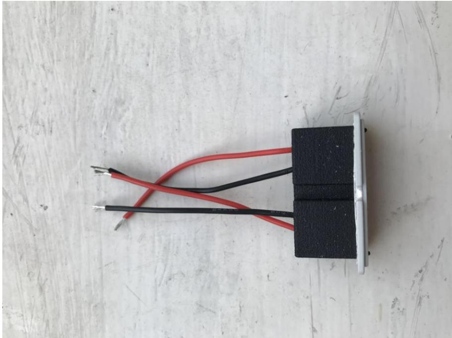
The picture above shows the device connector housing inserted into the PIL Box end plate slot created earlier. Note the device connector base plate location lugs poking just past the PIL Box end plate. When dry, place the assembly in the vice and locate & glue the device connector base plate on to the front of the PIL Box end plate.
