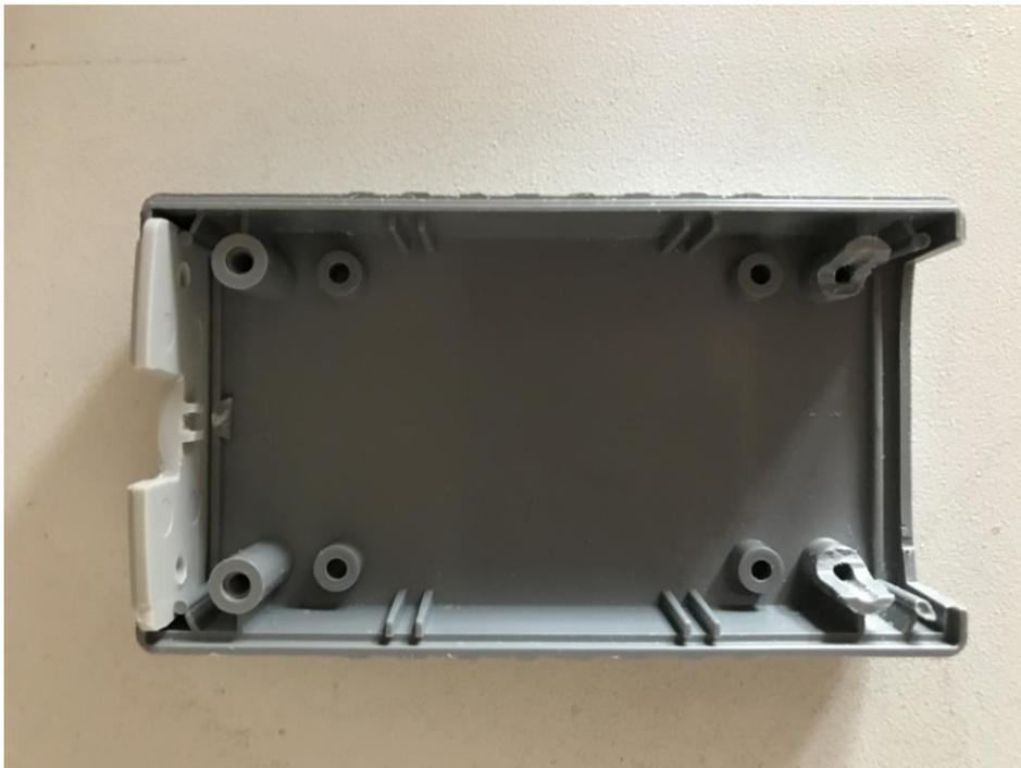
The picture above shows the screw pillars (right) cut away to allow space for the device connector housing, the PCB still rests nicely on the smaller posts.
