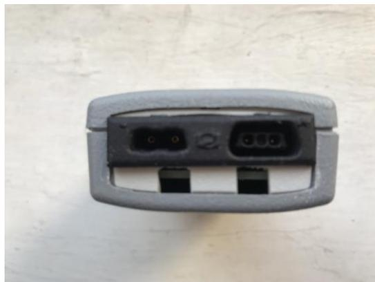
The picture above shows the device connector fully assembled in the PIL Box. HP-IL cables can now be plugged directly into the PIL Box (the original end plate cut outs for the wires can still be seen)! The picture for some reason looks a bit wonky this may be because the case at this end is no-longer clamped down with screws, but it looks much better in real life!
