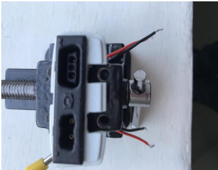
The picture above shows the device connector base plate fixed to the PIL Box end plate with the device connector housing behind (mounted in the modelling vice for display purposes). When dry, remove the PCB from the case and solder the device connector wires to the back of the PIL Box PCB then reassemble device connector & PCB back into the case ensuring the wires go past the PCB sides.
