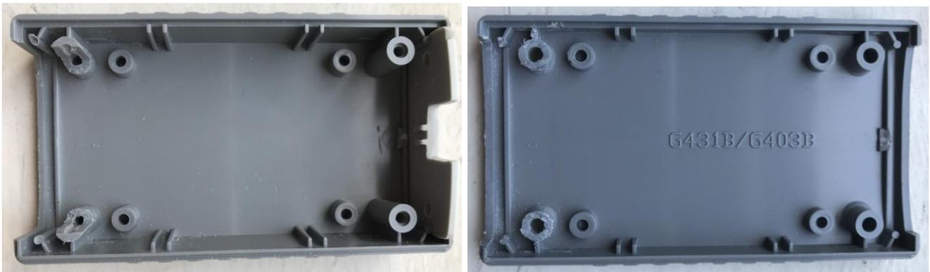
The pictures above show the 'long' screw posts (left picture) cut diametrically in parallel to the housing walls down to the level of the adjacent housing 'hole' and the 'smaller' screw posts in the 'upper' half of the housing cut off completely down to the level of the adjacent housing hole (right picture) and were then 'cleaned up' with a model makers file.
