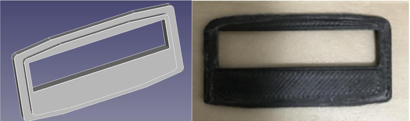
The pictures above show the 3D design that includes a step or 'lip' that fits in the PIL-IO housing groove and a slot that the HP-IL connector fits in.
