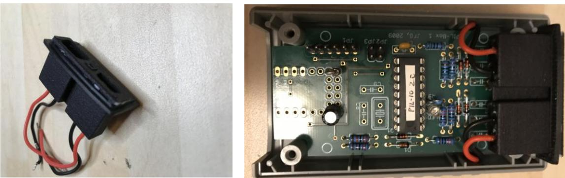
The pictures above show the bonded connector assembly (left) ready for mounting into the PIL-IO housing. The connector leads are soldered to the underside of the PCB and positioned to prevent trapping by the housing walls as shown in the right picture.
