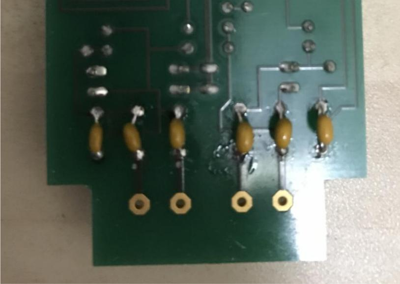
The picture above shows the HP-IL input end of the PCB with the input capacitors re-located on the underside of the PIL-IO PCB. This then completes the housing/PCB modifications.
